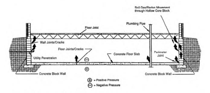
Figure 1-4a. Typical radon entry routes in concrete block basement walls.
