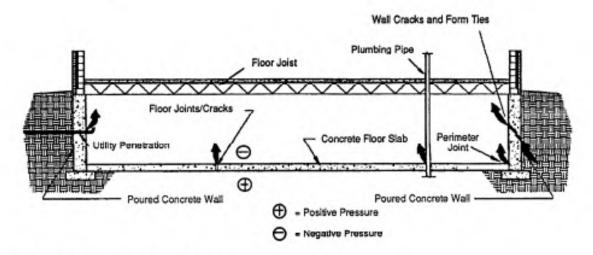
Figure 1-3. Typical radon entry routes in slab-on-grade construction.
