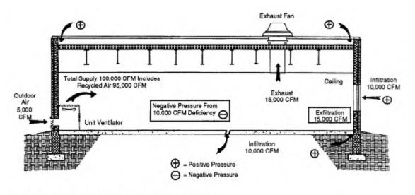
Figure 2-9. Example of building depressurization with HVAC system.
