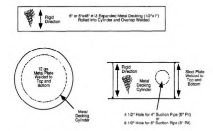
Figure 2-13. Smaller subslab suction pit.
