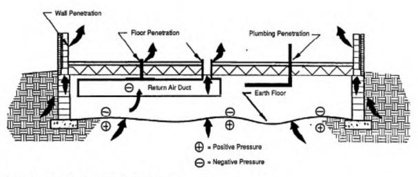
Figure 1-5. Typical crawl space foundation entry routes.
