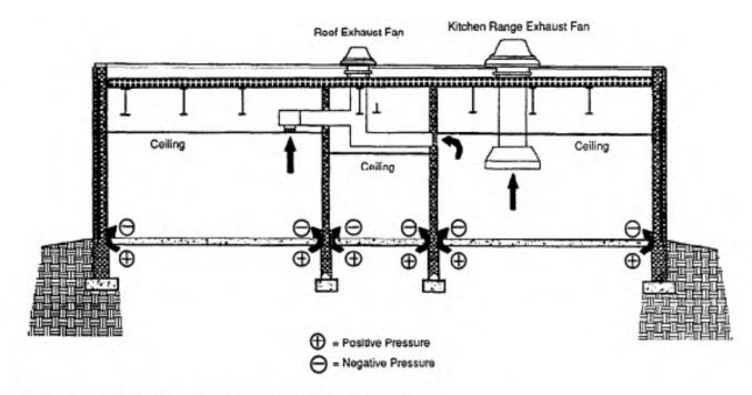
Figure 1-2. Examples of negative pressure sources in a typical building.
