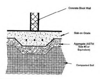
Figure 2-2b. Thickened slab footing. Not to scale.
