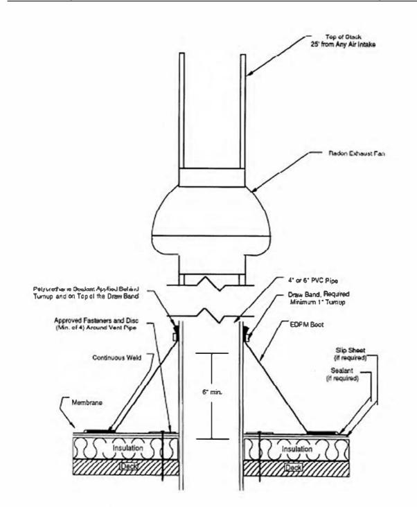
Figure 2-6. Sealing pipe penetrations through roof. Not to scale.
