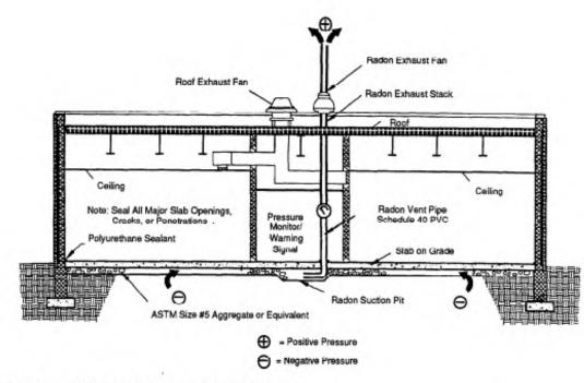
Figure 2-1. Typical substab depressurization system. Not to scale.
