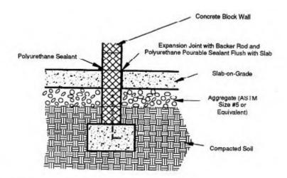
Figure 2.2a. Interior footing/foundation wall. Not to scale.
