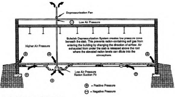
Figure 1-6. Subsiab depressurization theory.
