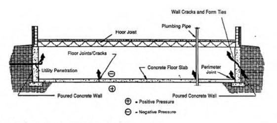
Figure 1-4b. Typical radon entry routes in poured concrete basement walls.
